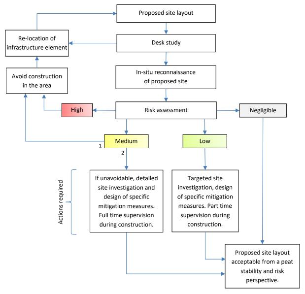
Figure 1-2: Workflow of the PSRA methodology for the acceptability of the proposed site layout.
