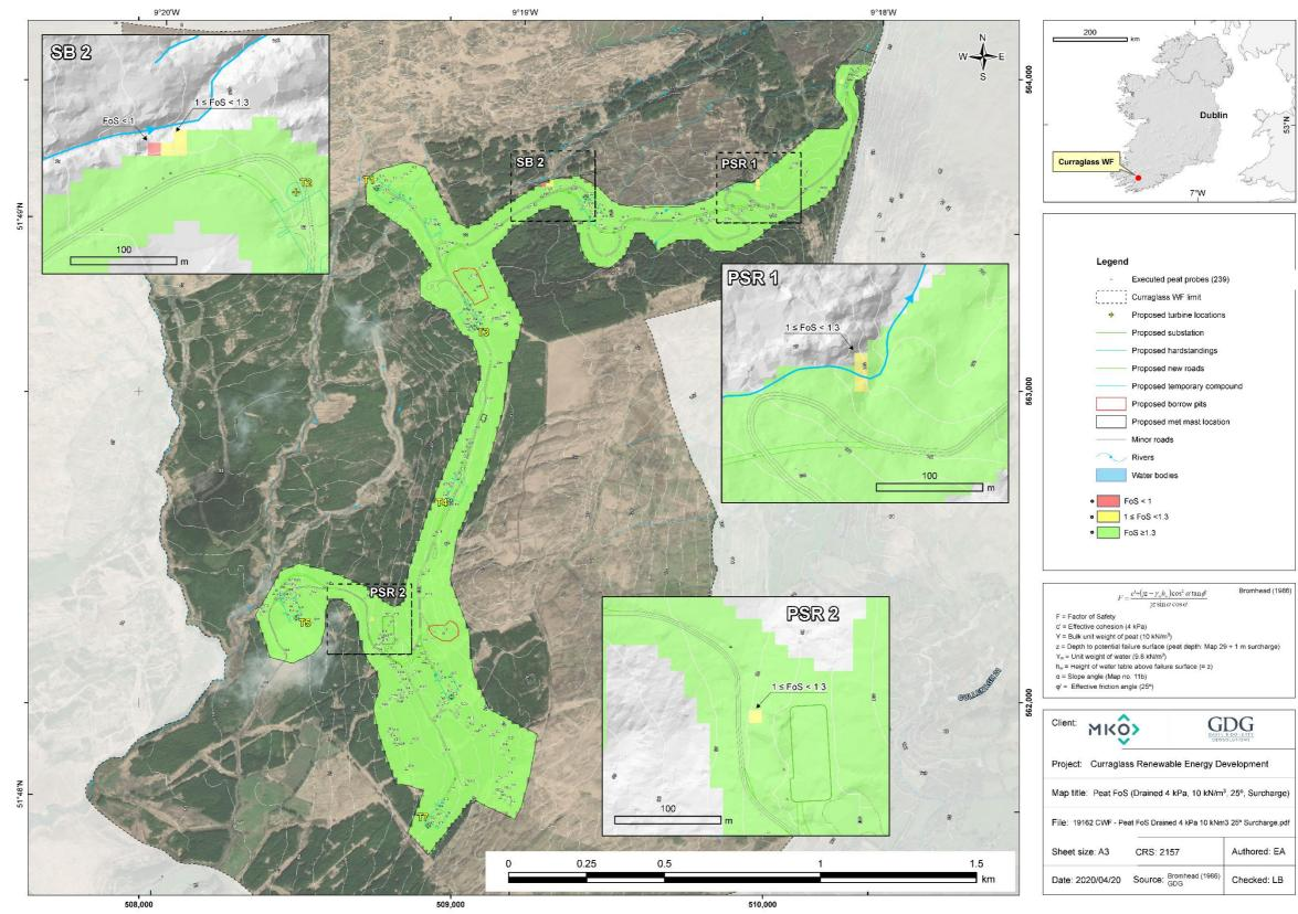
Figure K-4: FoS for drained conditions and surcharge of 1 m (i.e. 10 kPa).
