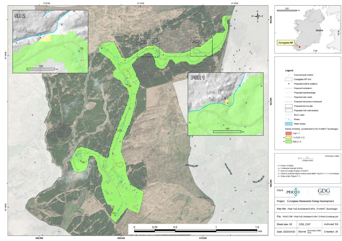
Figure K-2: FoS for undrained conditions and surcharge of 1 m (i.e. 10 kPa).
